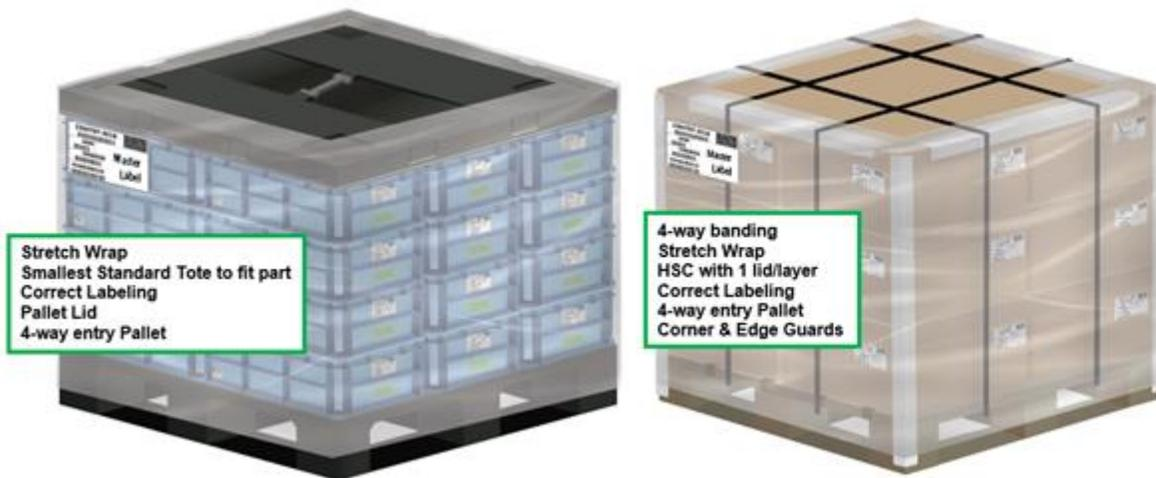
Band pallets through openings with plastic banding:
